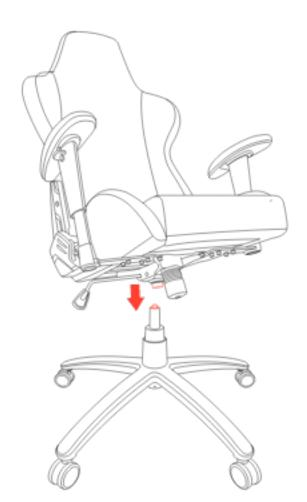
Insert top of the hydraulic lift cylinder into the mounting hole on the control unit, then place the chair upright.
