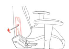
Install the side covers and tighten the bolts to secure them in place. (Place the cover designated "R" on the side of the chair with the lever.)
